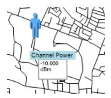
If a GNSS receiver is active, and you are using a geo-referenced map, a single measurement is placed at the current GNSS coordinates.
