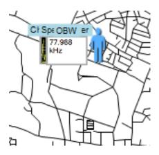
**NOTE.** The number of measurements that can be placed on a map is limited to 200. When the limit is reached, RSA Map shows a message stating that the limit has been reached, and discards any following measurements. Select File > Save As to save the map and measurements to a file, or select File > Clear All Measurements to clear the map and resume adding measurements to the map.
