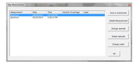
**4.** Click **View in Instrument** to show the measurement screen for the selected measurement on the Host Instrument. Select **Tools** > **RSA Map** on the Host Instrument to return to the RSA Map screen.
