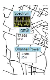
**NOTE.** Moving a measurement icon results in the geographic location data for the moved measurement icon being changed to that of the map location the measurement icon is moved to.
